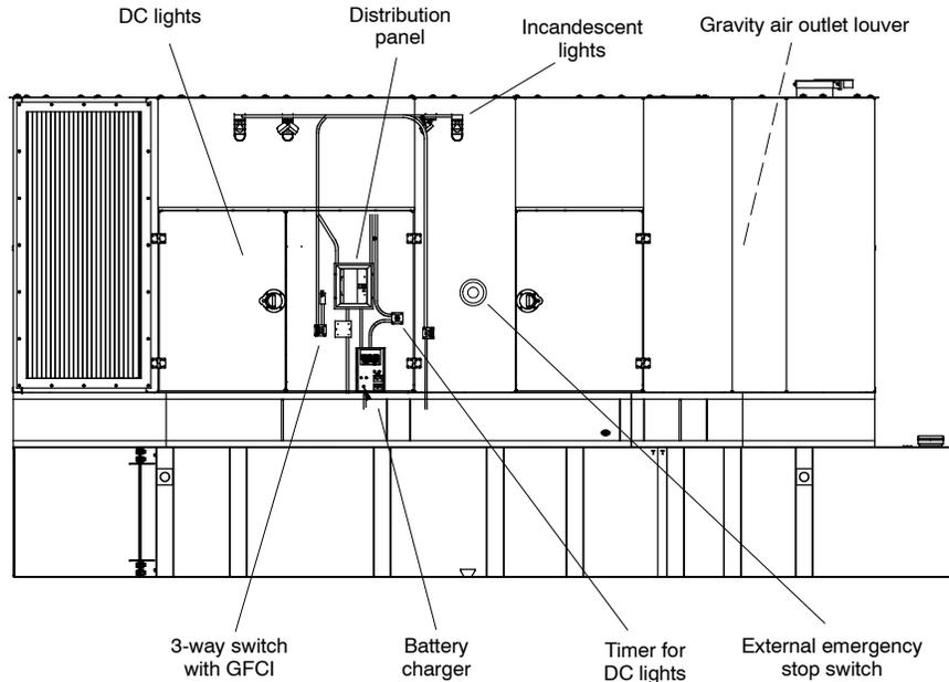
**Note:** Enclosure heater and ventilation fan not shown.
